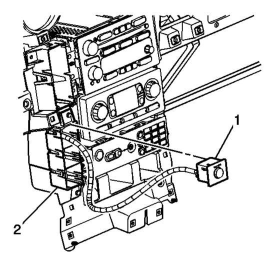
Fig. 19: Traction Control Switch & I/P Assembly Courtesy of GENERAL MOTORS CORP.
