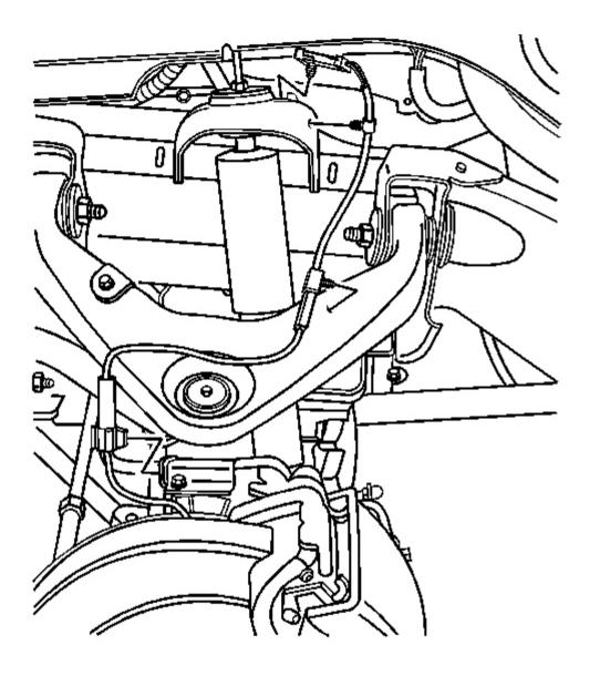
Fig. 13: Front Wheel Speed Sensor Cable Courtesy of GENERAL MOTORS CORP.
