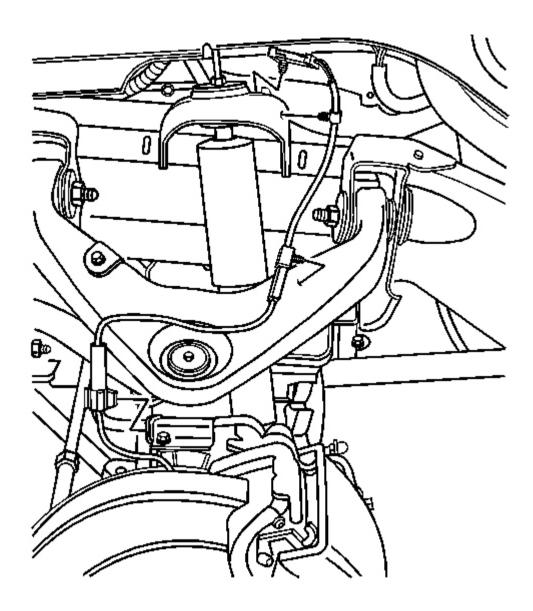
Fig. 16: Front Wheel Speed Sensor Cable Courtesy of GENERAL MOTORS CORP.
