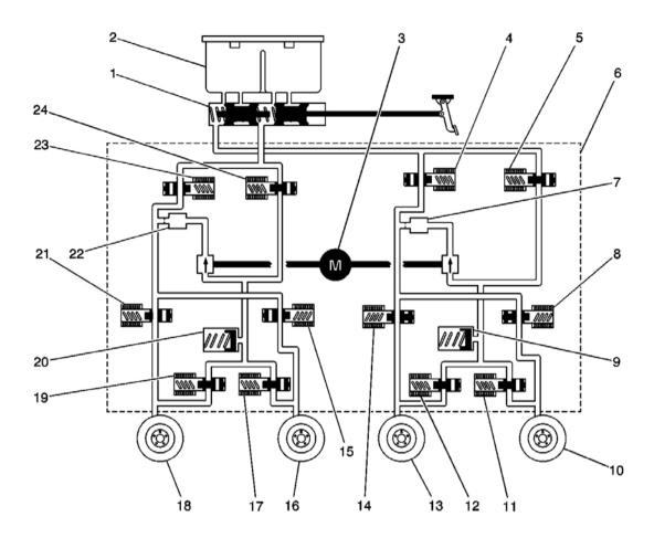
Fig. 24: BPMV Hydraulic Flow Courtesy of GENERAL MOTORS CORP.
