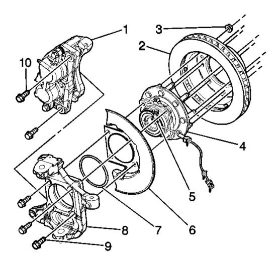
Fig. 14: Wheel Hub And Bearing (RWD, 25/35 Series) Courtesy of GENERAL MOTORS CORP.
