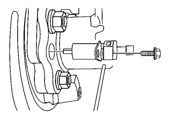
Fig. 17: Rear Wheel Speed Sensor & Shim Courtesy of GENERAL MOTORS CORP.
