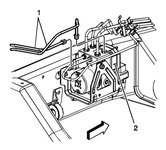
Fig. 8: Rear Brake Pipes & BPMV Courtesy of GENERAL MOTORS CORP.
