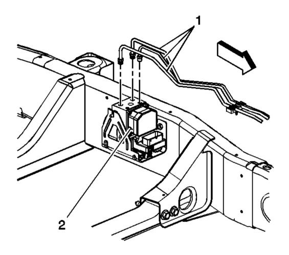
Fig. 10: Identifying BPMV Courtesy of GENERAL MOTORS CORP.
