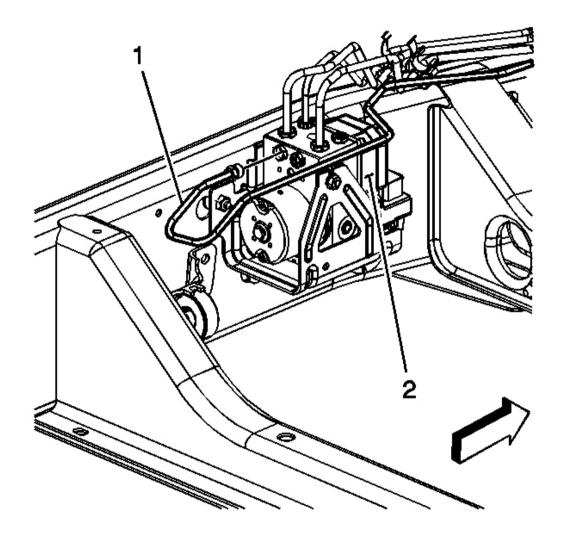
Fig. 12: Right Front Brake Pipe & BPMV Courtesy of GENERAL MOTORS CORP.
