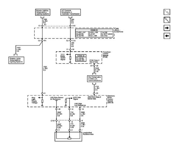
Fig. 2: Stoplamp Switch and Longitudinal Accelerometer Inputs Courtesy of GENERAL MOTORS CORP.
