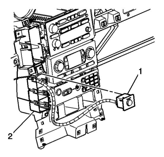
Fig. 20: Traction Control Switch & I/P Assembly Courtesy of GENERAL MOTORS CORP.
