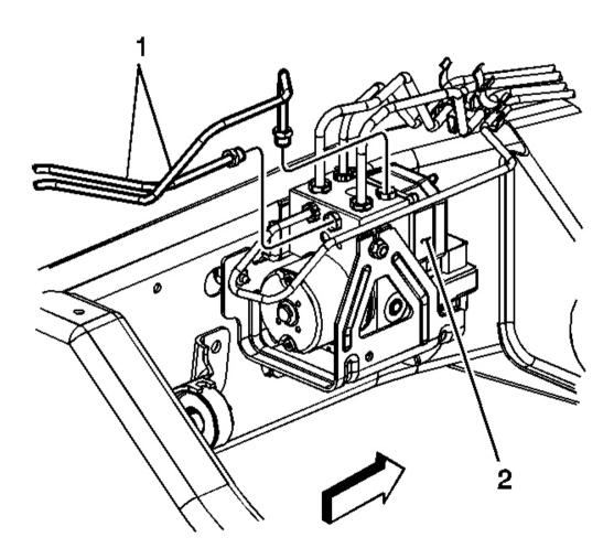
Fig. 11: Rear Brake Pipes & BPMV Courtesy of GENERAL MOTORS CORP.
