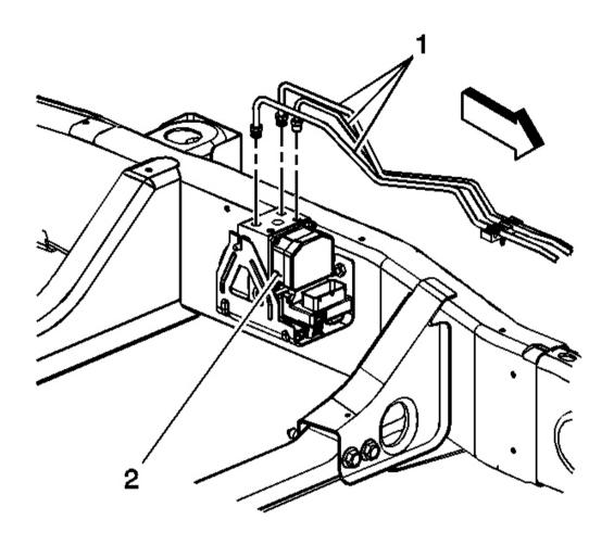
Fig. 9: Identifying BPMV Courtesy of GENERAL MOTORS CORP.
