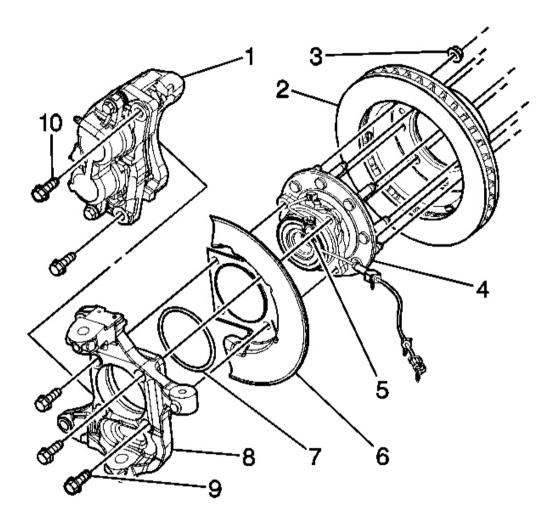
Fig. 15: Wheel Hub And Bearing (RWD, 25/35 Series) Courtesy of GENERAL MOTORS CORP.
